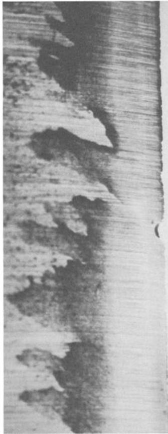
FIG. 4— Photomicrograph of cutting edge, revealing cutting surface and defects in blade.
